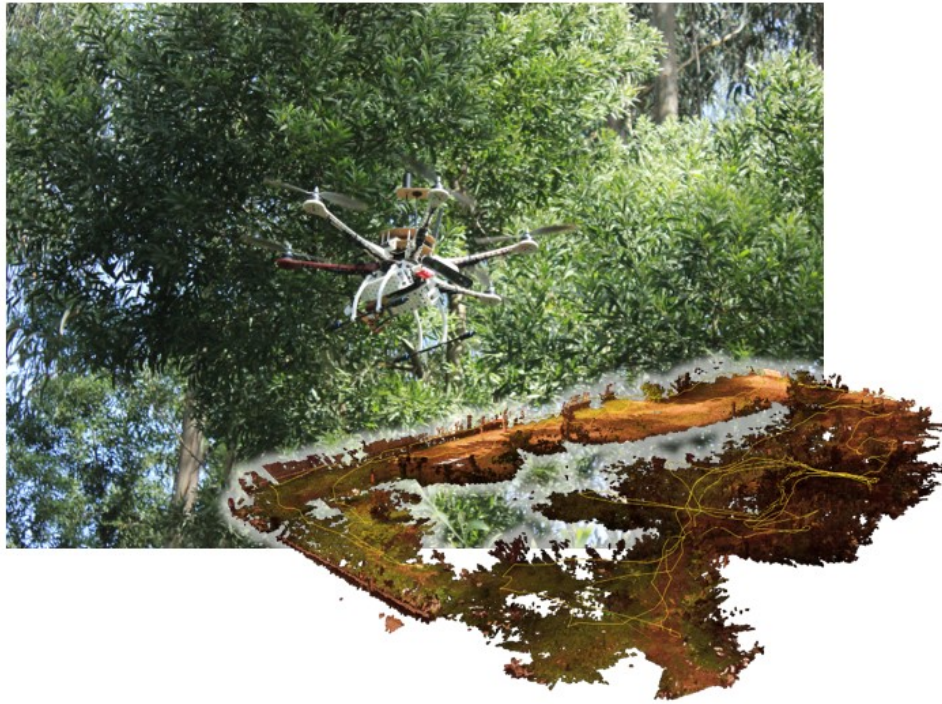
Figure 5: A single OpenSwarm UAV performing SLAM in the forest.
